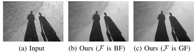
Fig. 2. Example result of our approximate global mode filter ( \mathcal{F} is box filter) and dominant-mode filter ( \mathcal{F} is Gaussian filter).
